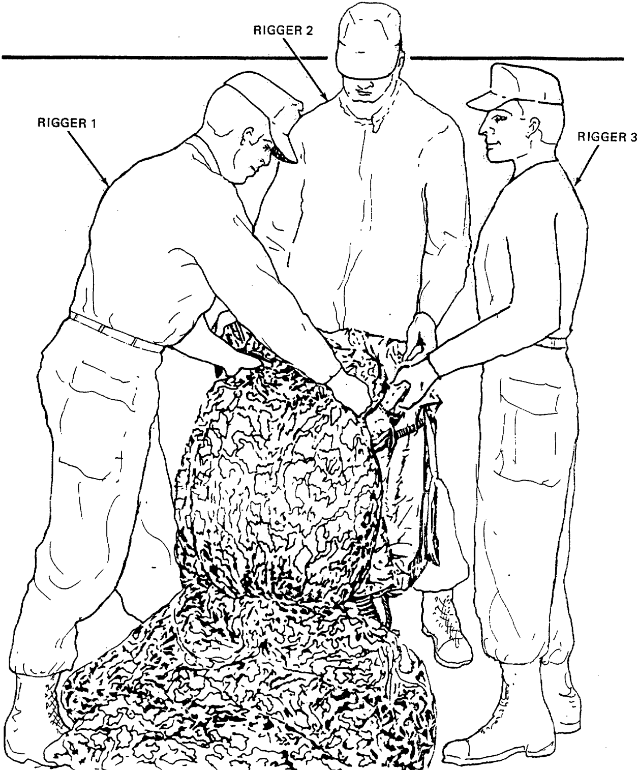
Figure 2-79. Stowing the Canopy Into the Deployment Bag .
