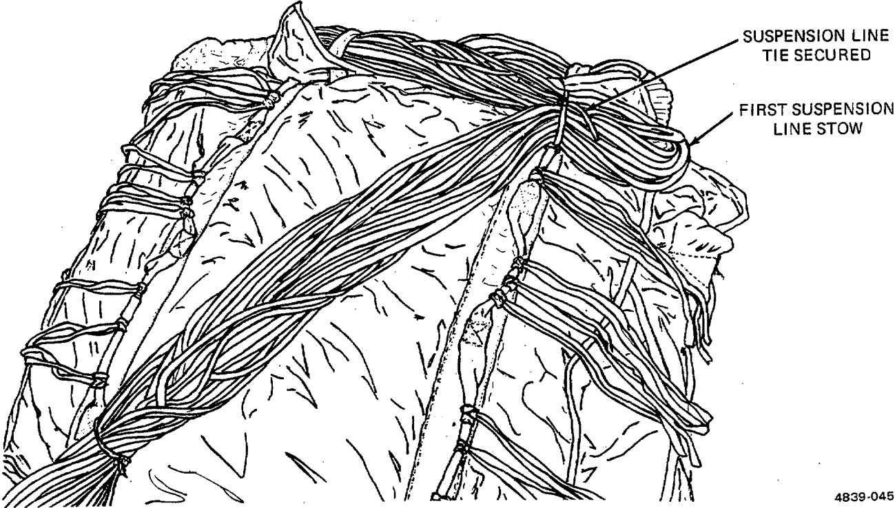
Figure 2-36. First Suspension Line Stow Completed.
